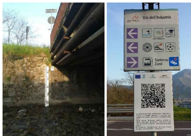
Figure 1. Photos showing staff gauges and QR codes used in the WeSenseIt project.
